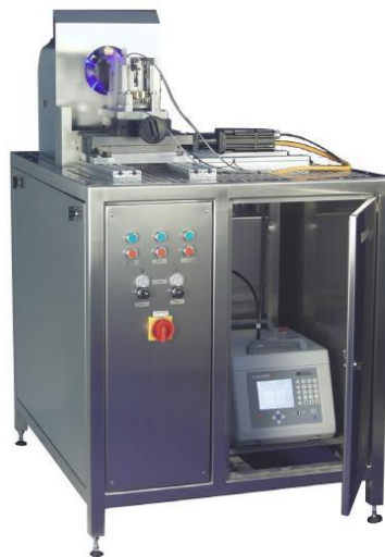
Figure 2 Cleanroom-suitable material test bench "Material Inspec" developed by Fraunhofer IPA with module for ball-on-disk test. The module can be replaced if necessary with the module for reel-on-disc test.
